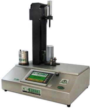
The Front End Station provides a new alternative for manual front end measurements on trimmed 2-piece cans.
