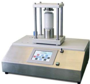
The easy-to-use AXL-3050 tester measures the axial load resistance of beverage cans, and provides a force over time diagram.
