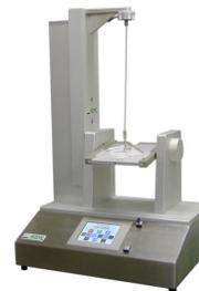
Buckle Tester for Loose Ends
