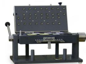
This enamel rater connects to a variety of attachments allowing for rapid testing of up to 16 cans, can ends, crowns, or twist-off caps.
